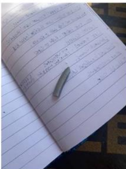
Foreign body from the plastic pot broken off (22mm).
