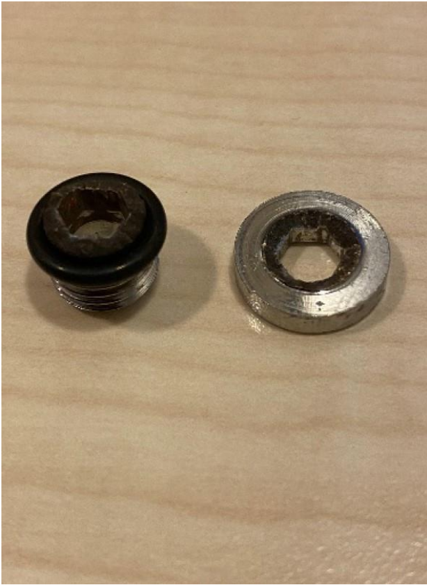
The two pieces of the failed blanking plug
