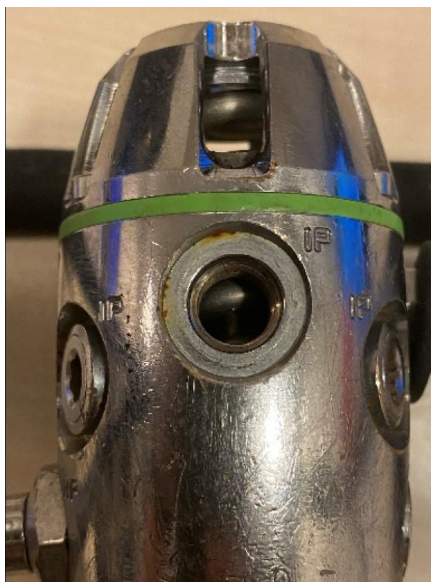
Regulator with 1st stage with low pressure port identified
